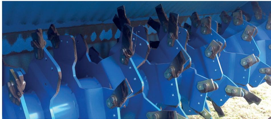
By means of our patented roller pendulum system, you can easily control the operating depth. As a unique bonus, we have provided the scarifying machine with a hydraulic adjustable cover. This is ideal when you are required to scarify near the edges and corners of a pitch.
