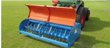
Since you can hydraulically adjust the pressure roller, you can execute both operations separately or you can aerate and level at the same time. The combination of operations contributes to the reduction of the CO2 emissions, and benefit the transition towards chemical free management of your grass.
