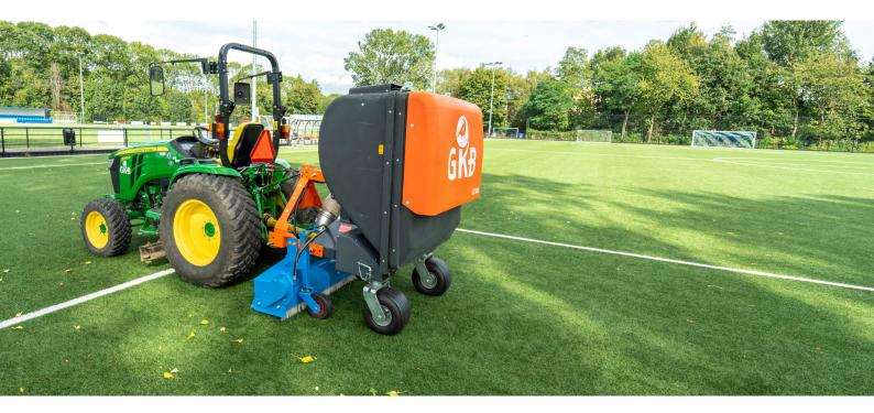
The Leaf-Clean is a ideal vacuum machine for vacuuming three leaves, small branches or cut grass on artificial grass fields, hybrid fields and nature fields. Because of the forward movement of the tractor, the leaves/ branches come under the shaft of the nozzle. The leaves are held under the shaft by the brush hole at the back and the partitions at the side.
