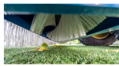
The brush sweeps the leaf/branches in one heap. When the pile is high enough, the rotating brush takes some of the swept heap and throws it into the air shaft. The air stream picks up the leaves, twigs or clippings and transports them to the container.
