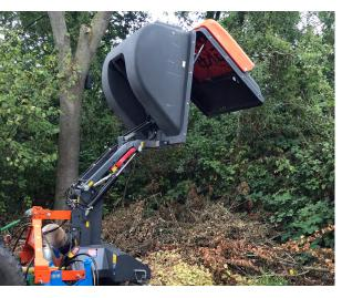
The vacuum machine has a capacity of 1.050 liters. When the collection box is full, it can easily be emptied. By means of a lifting function the operator can easily throw the leaves into a container.
