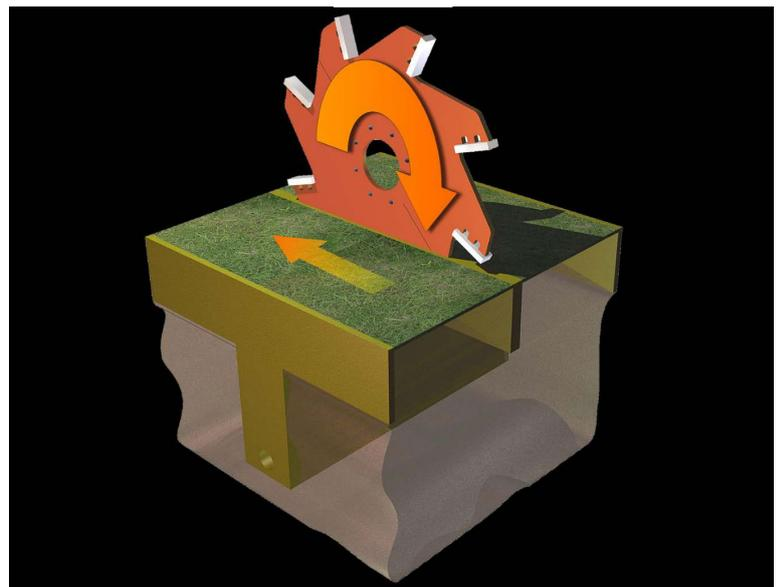
The Drainmaster is also available in a model with a working width of 85 cm. It creates two trenches instead of the three trenches that the DM150 creates. In addition, you can operate the DM850 with a tractor with at least 90 hp.
