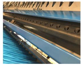
The seed dosing system gives you the opportunity to divide the amount of seed accurately on the soil. It is possible to seed from 3 up to 50 grams per square meter. Using the lever behind the seed hopper you can adjust the opening for the seed dosing.
