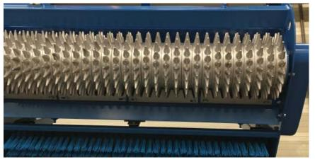
The conical spike rollers produce 1500 holes per square meter, opening up the soil and the seed falls behind the first roller. The spike rings are loosely mounted on a rotor tube so they can move separately, enabling you to make turns without damaging the grass. Behind the rollers, the two brushes sweep seed and topdressing, with the first brush being adjustable for pressure and the second following the contours.
